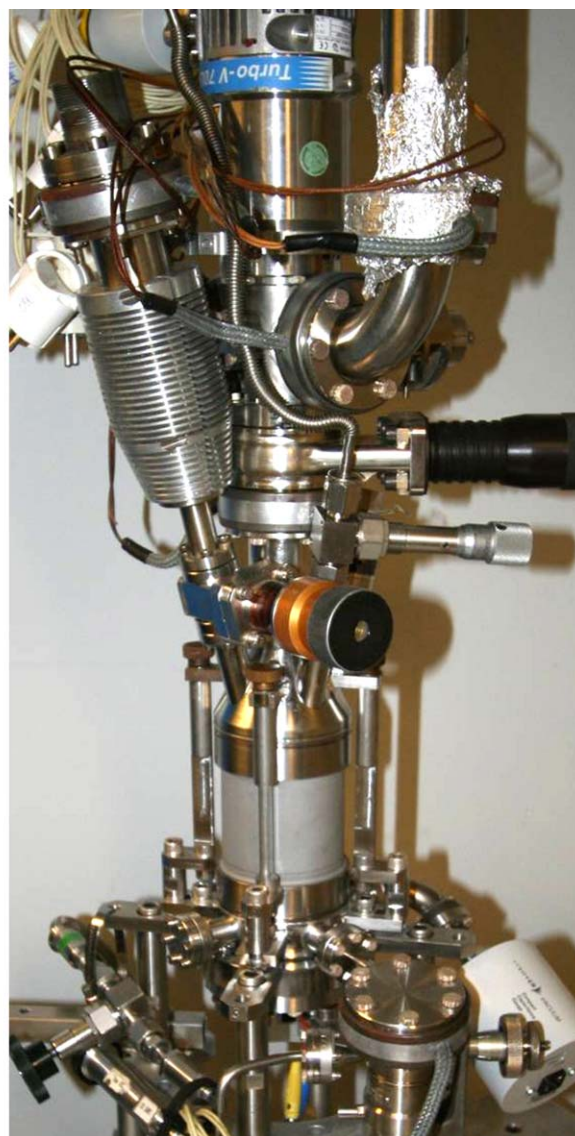
Fig. 2. Left: a schematic drawing of the high pressure batch reactor. The sample is represented as a red rectangle at the bottom. The incoming X-ray beam is represented as a solid red arrow, the outgoing beam is represented as dashed red arrows. Right: a picture of the batch reactor.
