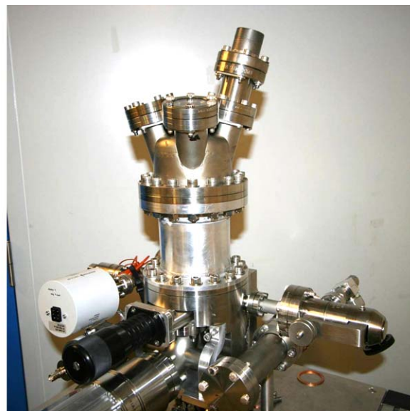
Fig. 3. Left: a schematic drawing of the batch reactor for harsh conditions. The sample is represented as a red rectangle at the bottom. Right: a picture of the reactor.
